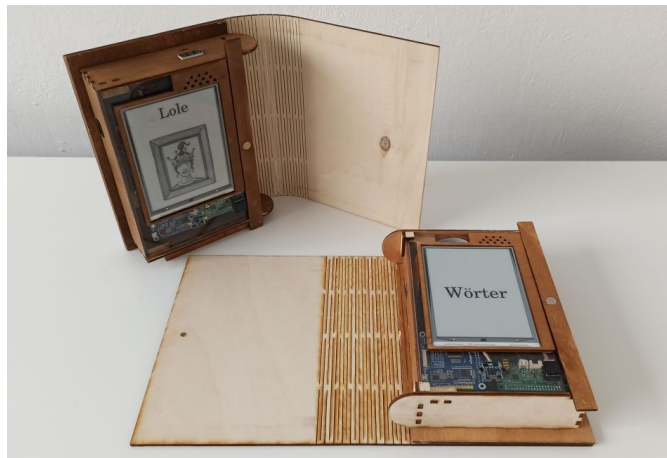
Figure 1: Left-hand and right-hand version 1 prototypes of Personal Primer (PP) artifact with integrated speech capabilities, e-ink displays and touchless gesture command & control interface.
